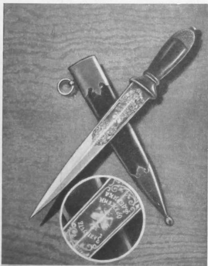
Fig. 11—Damascus steel dagger. The background is a photograph of the etched damask pattern of the blade, magnified 8 times (Ziegler, Mining and Metallurgy , v. 20, 1939, p. 60).
