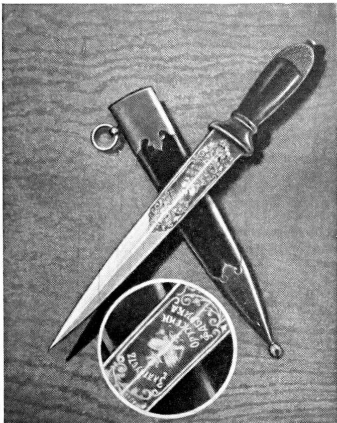
Fig. 11—Damascus steel dagger. The background is a photograph of the etched damask pattern of the blade, magnified 8 times (Ziegler, *Mining and Metallurgy*, v. 20, 1939, p. 69).
